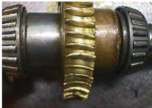
Worn Bronze Worm Wheel — Typical Sliding Friction Damage
